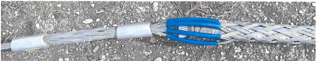
Photo 4 Pulling swivel, "Socks" and "Bug" used for stringing test
