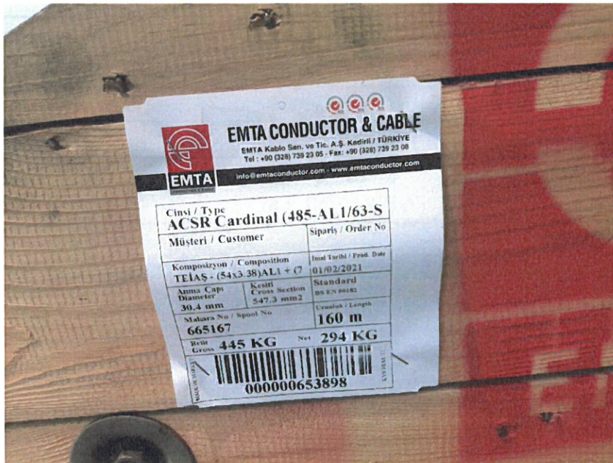
Photo 2 Label and markings on the surface of the Drum
